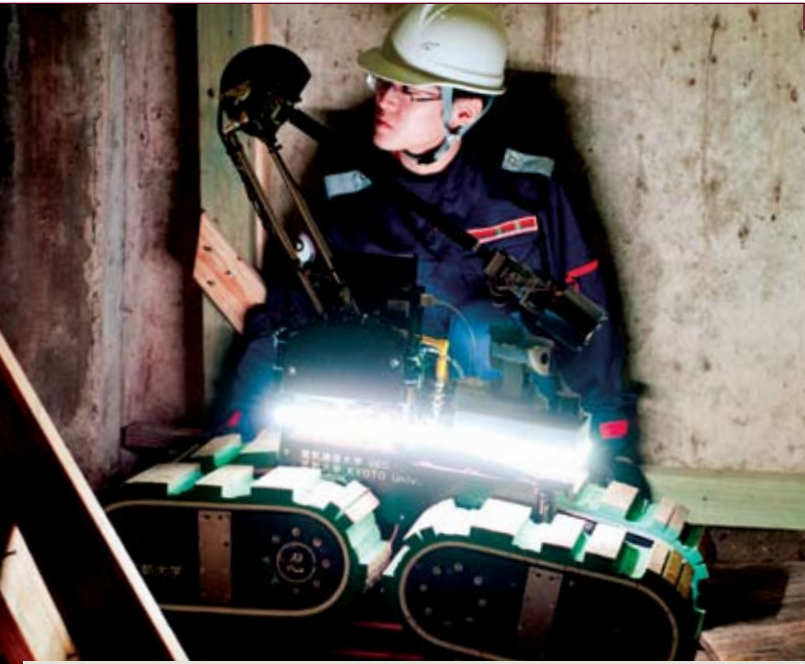
EXPLORING DISASTER The KOHGA3 robot is equipped with three CDC cameras, a thermal camera, laser scanner, LED light, altitude sensor, gas sensor and one-meter long robotic arm. The International Rescue Systems Institute is using KOHGA3 to explore damaged structures in the aftermath of the earthquake and tsunami.
