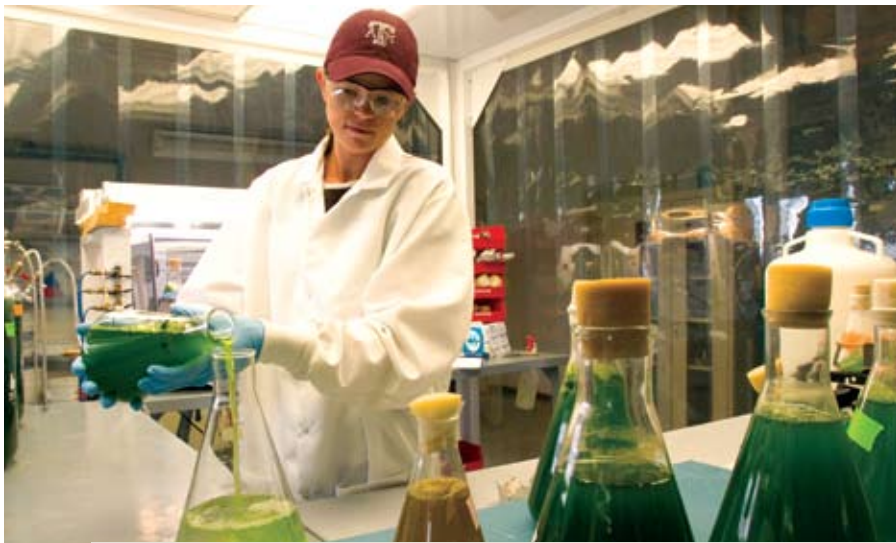
SCALING UP Researchers in Pecos, Texas, propagate microalgae in laboratory-scale vessels testing various species for high growth and lipid accumulation before scaling up to outdoor raceways.
